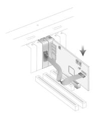
Figure 2-4: Installing the joystick port
